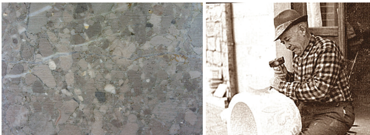
Figure 5 – Example of a slab of Breccia Irpina (on the left) and a worker of the stone (on the right).
