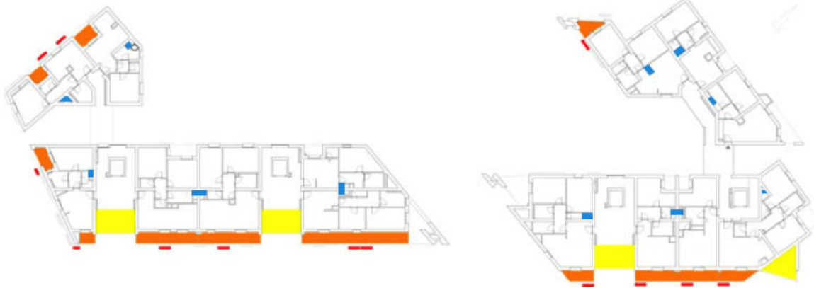
Figure 10 – Building plan with passive solar systems: in yellow the common six-floor sunspaces that provide preheated air for apartments in winter; in orange the private single-floor sunspaces for each apartment; in orange the Trombe-Michel walls that support the private sunspaces; in blue the ventilation tower that distribute air from sunspaces and from the underground slab.
