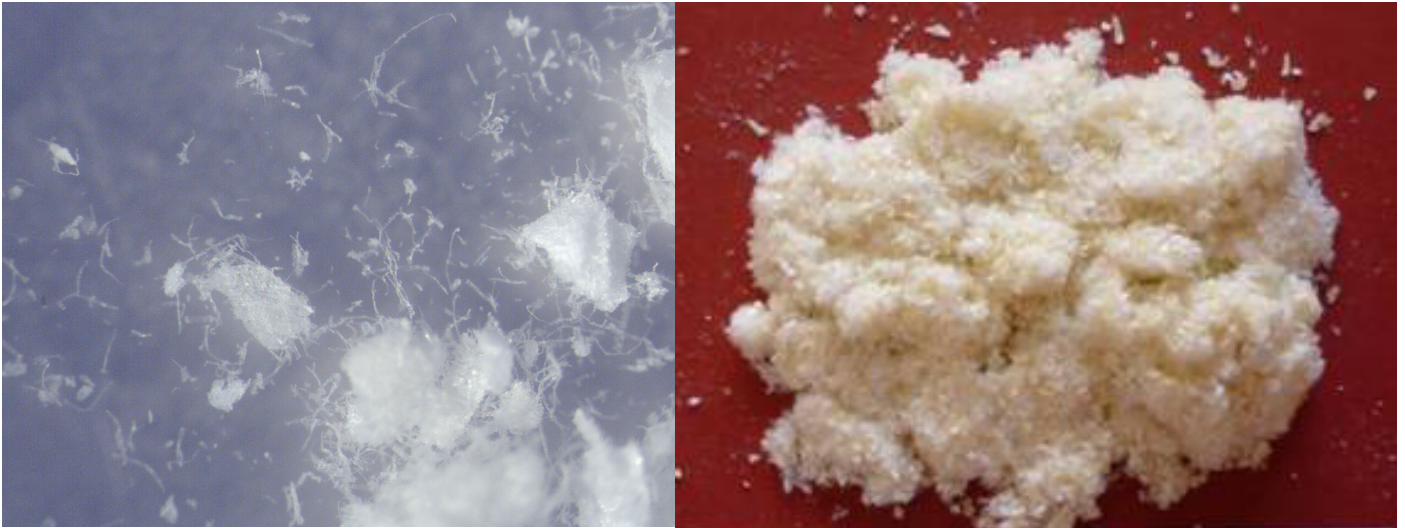
Figure 5 (on the left) and figure 6 (on the right): the charge obtained from knife mill with a sieve of 0,5mm observed with the stereomicroscope (fig. 5), the knife mill product (fig. 6).
