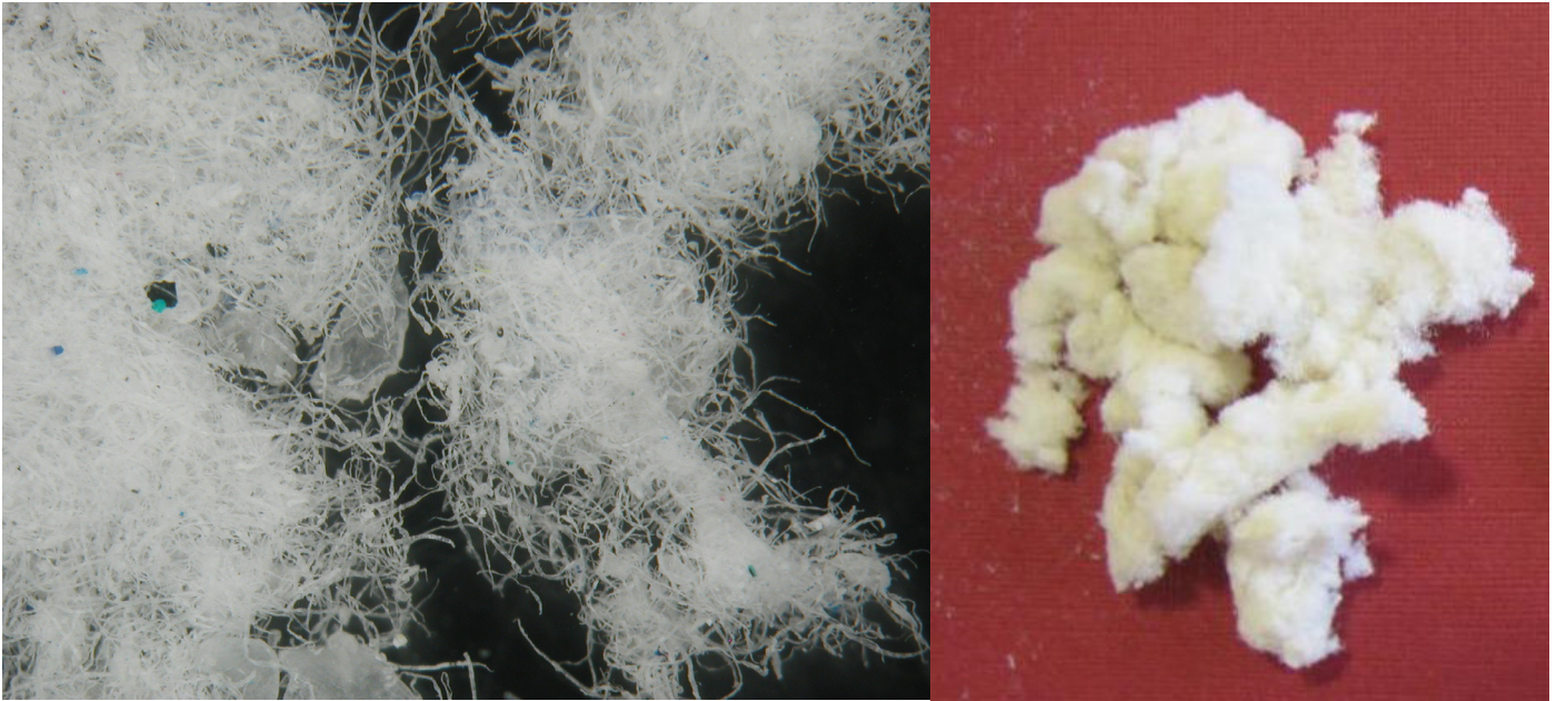
Figure 2 - (on the left) Micronized paper observed by stereomicroscope. Figure 3 (on the right) Micronized paper.
