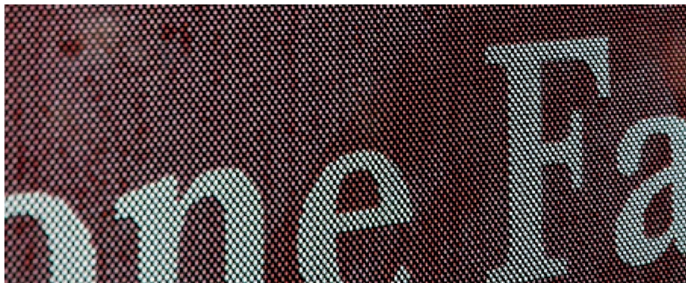
Figure 4 – Printed and perforated thin Film PV module CIS. Demo Object produced by Würth Solar and tested on La Spezia Castle according to the research program PVACCEPT.
