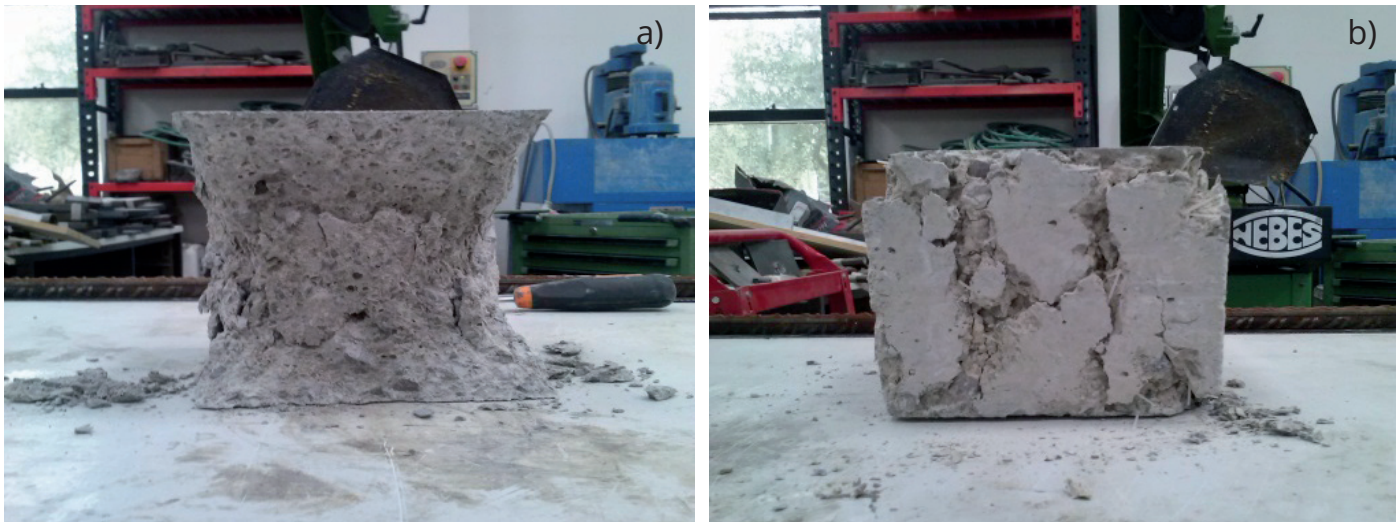
Figure 3 – a) Specimen without fibers; b) specimen with fibers.
