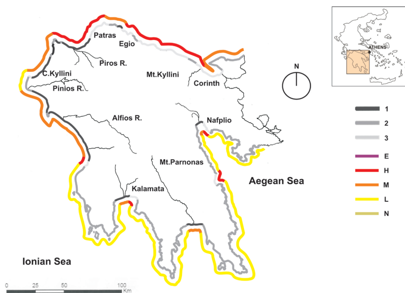
Figure 6 – Peloponnese (Greece): Map of the Coastal Geomorphologic Unit: 1, beach; 2, cliff; 3, technocoast and overall hazard along the coasts: E, extreme; H, high; M, average; L, low; N, negligible. The highest values are recorded primarily in the techno-coast UGC and the beach.
