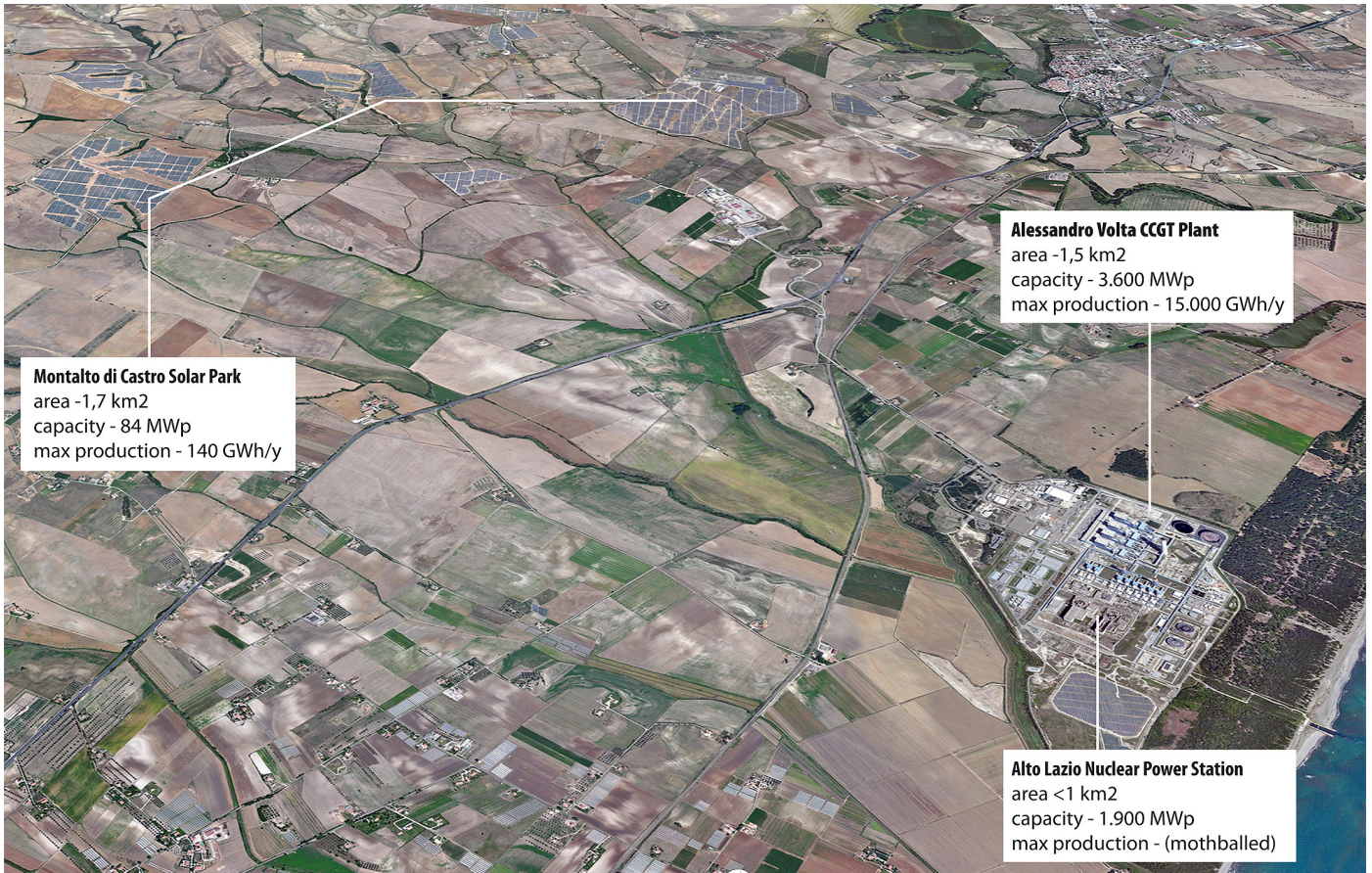
Figure 1 – Power generation technologies and land use. Comparing different magnitude scales in the emblematic context of Montalto di Castro (Italy).
