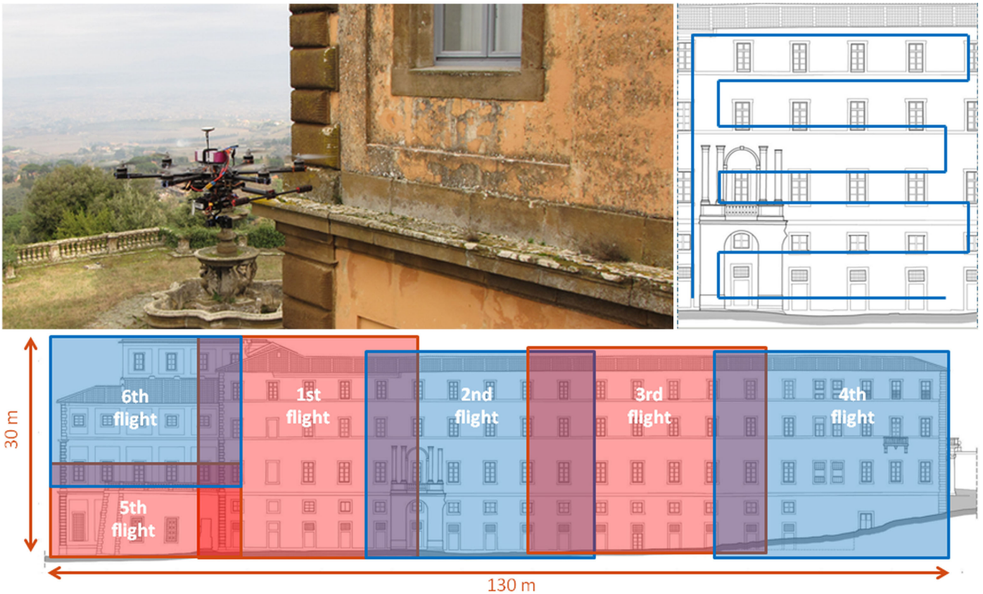
Figure 7 – Drone DJI A2 in flight equipped with digital video camera GoPro Hero 3+ (top-left) and flight project on the eastern external facade of the Manica Lunga (top-right and down).
