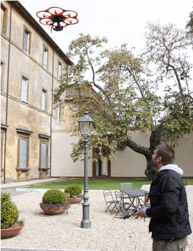
Figure 6 – Drone Aibotix X6 V2 in flight equipped with digital camera Olympus E-PL5 (left) and layout frame on the roof (right).
